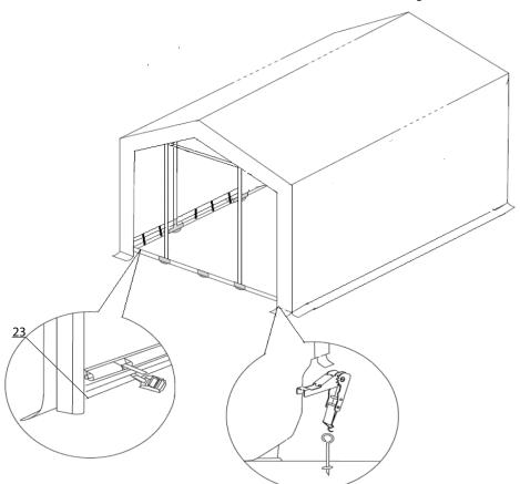
Spread the wall panel and door panel attach to framework by using the bangee cords clasping the frame to grommets that is construct over the wall panel and door panel to ensure stability. Also use the short pegs to fix the doors to the ground.
